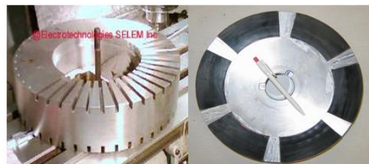
Fig. 2. Stator and rotor of the proposed machine.
