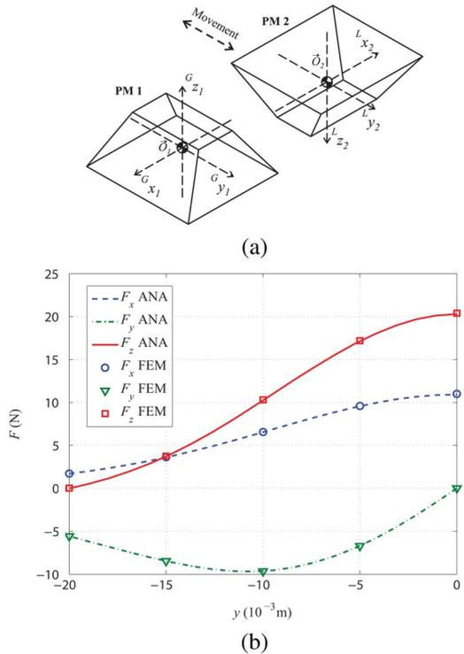
Fig. 6. Semi-analytical (dashed) and FEM results obtained for the interaction force between the PMs.
