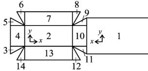
Fig. 3. Unfolded pyramidal frustum with fourteen segments.
