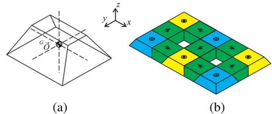
Fig. 1. (a) Pyramidal frustum and (b) Halbach array with pyramidal frusta.
