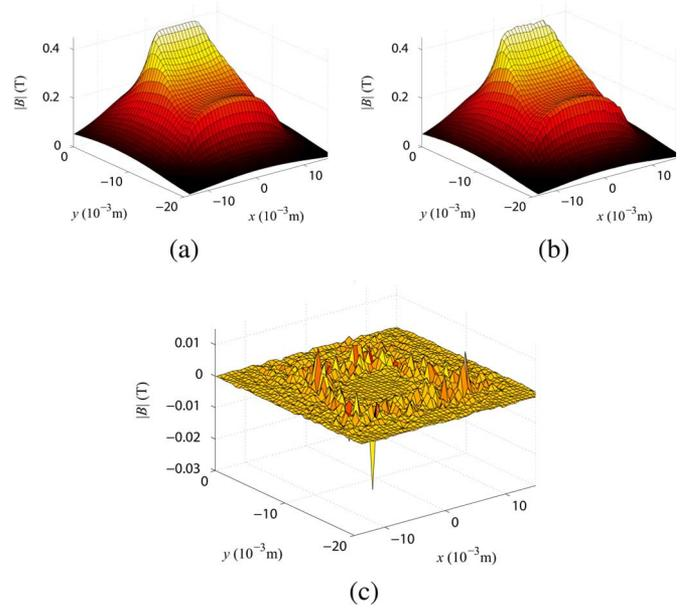
Fig. 5. Field calculation on a surface parallel to surface 10. Analytical results in (a), FEM results in (b) and their difference in (c).
