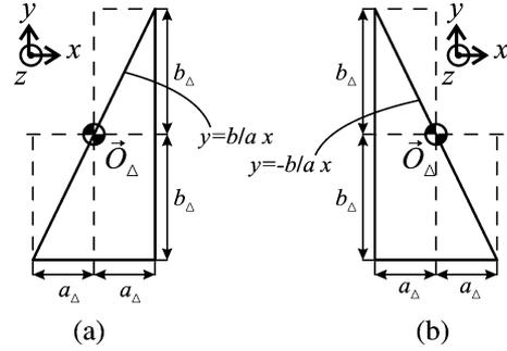
Fig. 4. Definition of the variables in triangular surfaces (a)  $\Delta 1$  and (b)  $\Delta 2$ .
