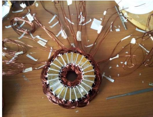
**Figure 2.** Distributed winding on stator steel core
