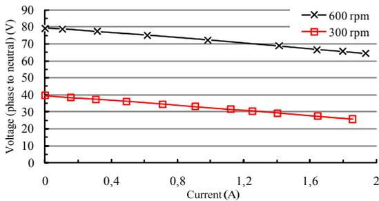
Fig. 12: Phase to neutral voltage versus current.
