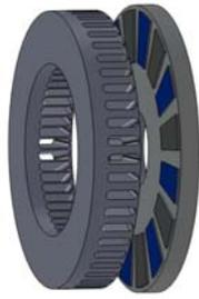
Fig. 1. Single stator-single rotor axial flux machine structure.
