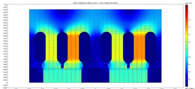
Fig. 7. Magnet flux density at the middle plane, under load condition.
