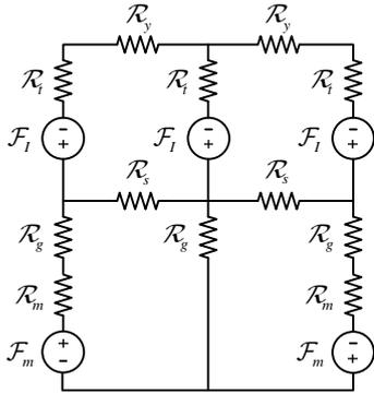
Fig. 4. Reluctance network over one pole pitch.
