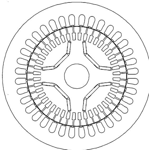
Fig. 3. Cross-sectional view of a four-pole LSPM.
