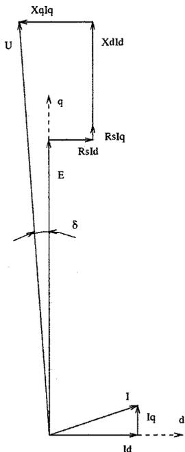
Fig. 2. Typical phasor diagram of a PMSM during no-load test. Note that the resistive voltage drops and the  $q$ -axis current are exaggerated for clarity.
