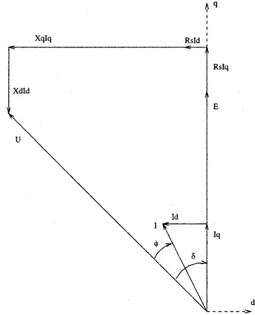
Fig. 1. Typical phasor diagram of a loaded PMSM fed directly from the mains.
