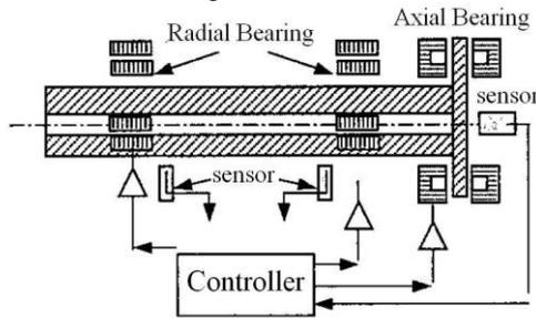
Fig. 7 Magnetic bearing
