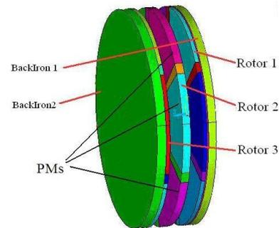
Fig. 3 Side view of high-speed axial-flux generators
