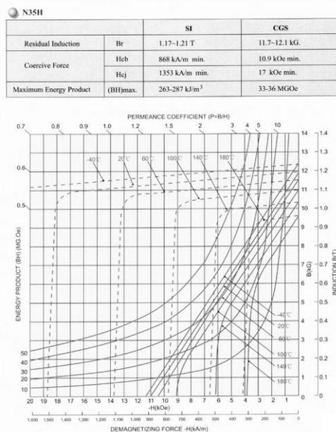
Fig. 4 Curves of N35H used in this machine
