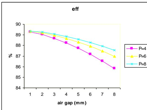
Fig. 11. Efficiency (%) vs. air gap (m)
