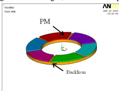
Fig. 5 View of a rotor of HSAFG
