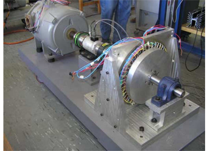
Fig. 7. Test lab setup for the 5 kVA, 8-pole AFPM prototype.
