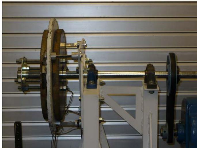
Figure 11. Laboratory setup for wind generator experiments
