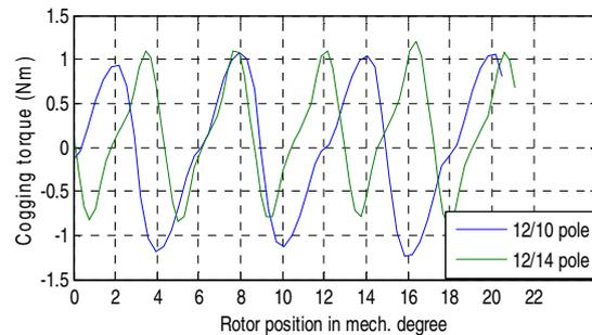
Fig. 14 Cogging torque of 12/10 and 12/14 pole FSPM machine.
