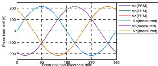
Fig. 11 Induced phase back EMF of 12/14 pole machine.
