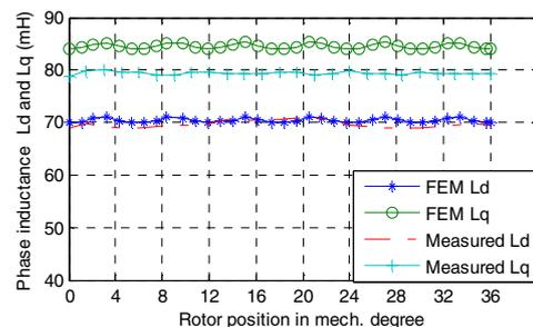
Fig. 15 Phase inductance of 12/10 pole machine.
