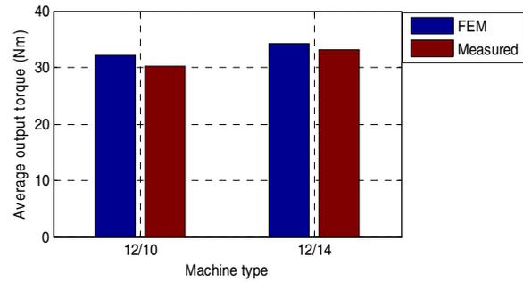
Fig. 13 Average output torque at the rated current.
