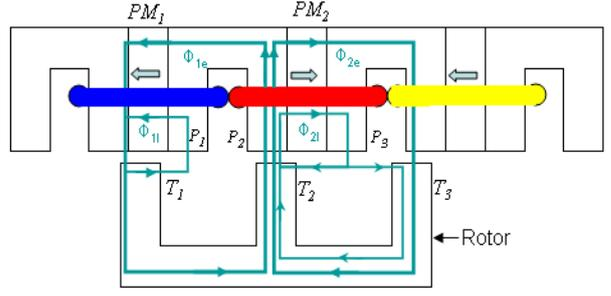
Fig. 5 Flux distribution in winding A1 when the total flux of A1 and A2 is maximum shown in Fig. 4.
