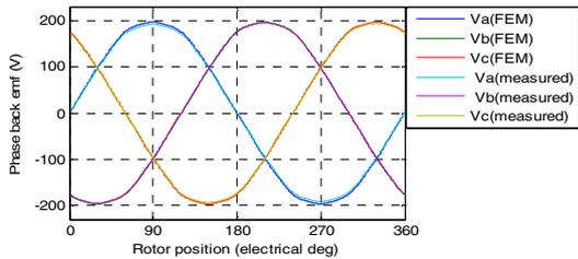
Fig. 10 Induced phase back EMF of 12/10 pole machine.
