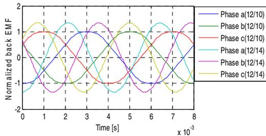
Fig. 6. Back EMF at no load condition.
