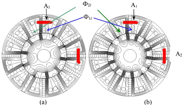
Fig. 4 Flux distribution at the maximum flux position of coil A (a) 12/10 pole machine (b) 12/14 pole machine.
