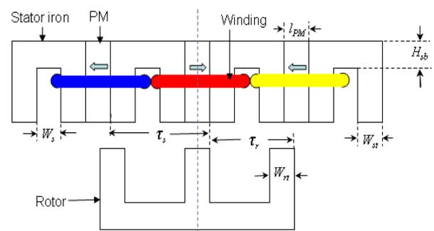
Fig. 2 Coil A1 at the zero flux position
