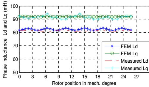
Fig. 16 Phase inductance of 12/14 pole machine.
