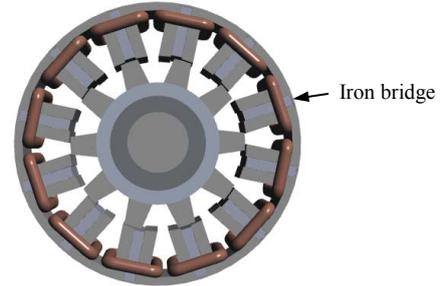
Fig. 8 3D view of the 12/10 pole prototype.
