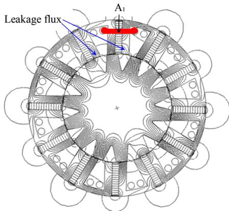
Fig. 17 Flux distribution in the 12/14 pole prototype machine at the maximum resultant flux position of coil A.
