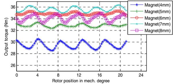
Fig. 18 Output torque with different magnet widths
