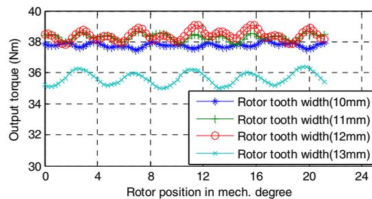
Fig. 20 Output torque with different rotor widths (fixed 7mm magnet).
