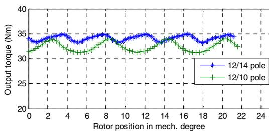
Fig. 12 Output torque from FEM calculations.
