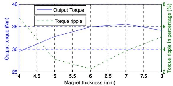
Fig. 19 Average torque and torque ripple (peak to peak).
