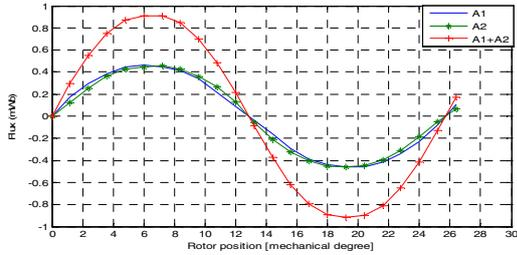
Fig. 3 Flux in coil A1, A2 and A1+A2
