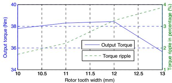
Fig. 21 Average torque and torque ripple in Fig. 20.
