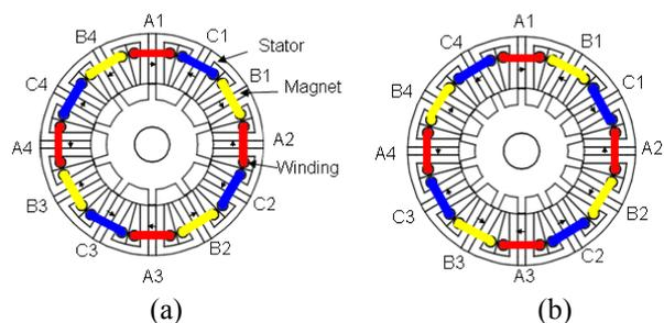
Fig. 1. (a) 12/10 pole (b) 12/14 pole machines.
