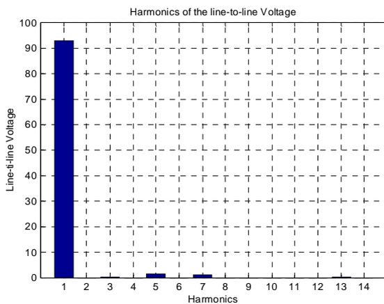
Fig 6: Line-to-line Voltage harmonic spectrum at 2000 [rpm].
