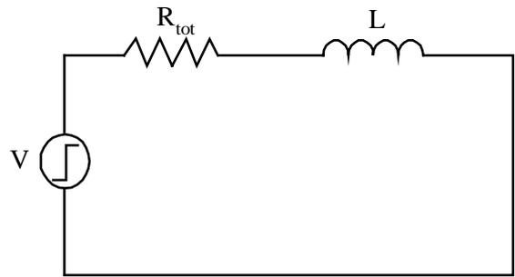
Fig 7: Machine one-phase representation with the rotor locked.
