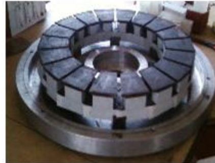
Fig. 6 Internal view of Stator
