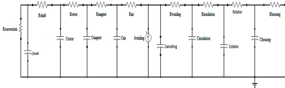
Fig. 3. Lumped-parameter model for the thermal analysis of the two aerospace actuators.
