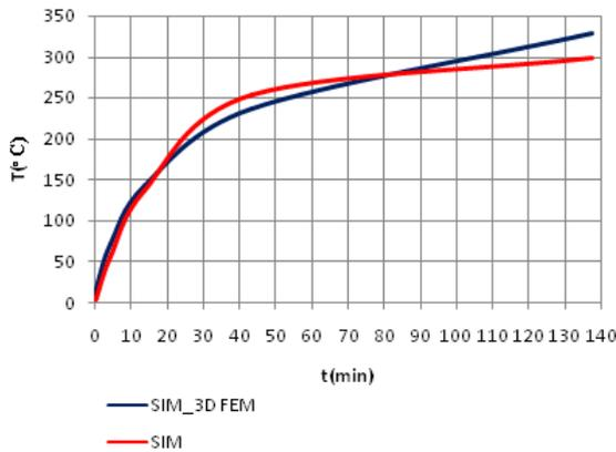
Fig. 4. Stator winding temperature variation of the actuators.
