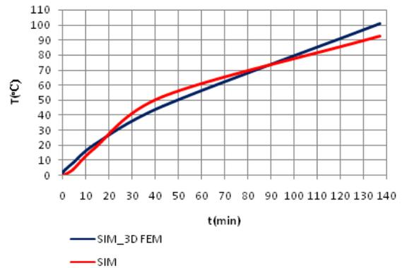
Fig. 5 Rotor temperature variation of the actuators.
