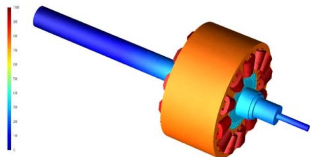
Fig. 2. PMSM temperature distribution at 2607 s.
