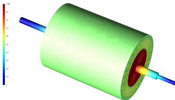
Fig. 1. IM temperature distribution at 2607 s.
